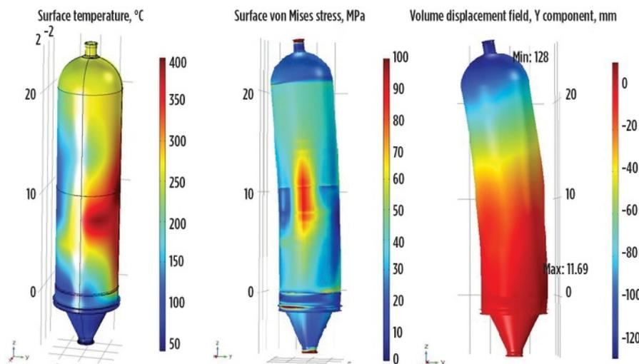
FIG. 3. Temperature map and corresponding stress map on the deformed shape of the coke drum at a selected moment during the cooling process.
