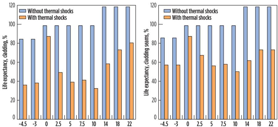
**FIG. 5.** Reduction in life expectancy of the cladding due to thermal shocks.
