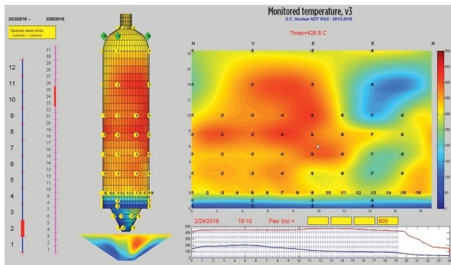
FIG. 1. A user interface with date, temperatures on the rotating model of the coke drum, unwrapped surface of the cylindrical parts (right) and cone (below 3D model), and a plot of extreme temperatures in time (low, right).
