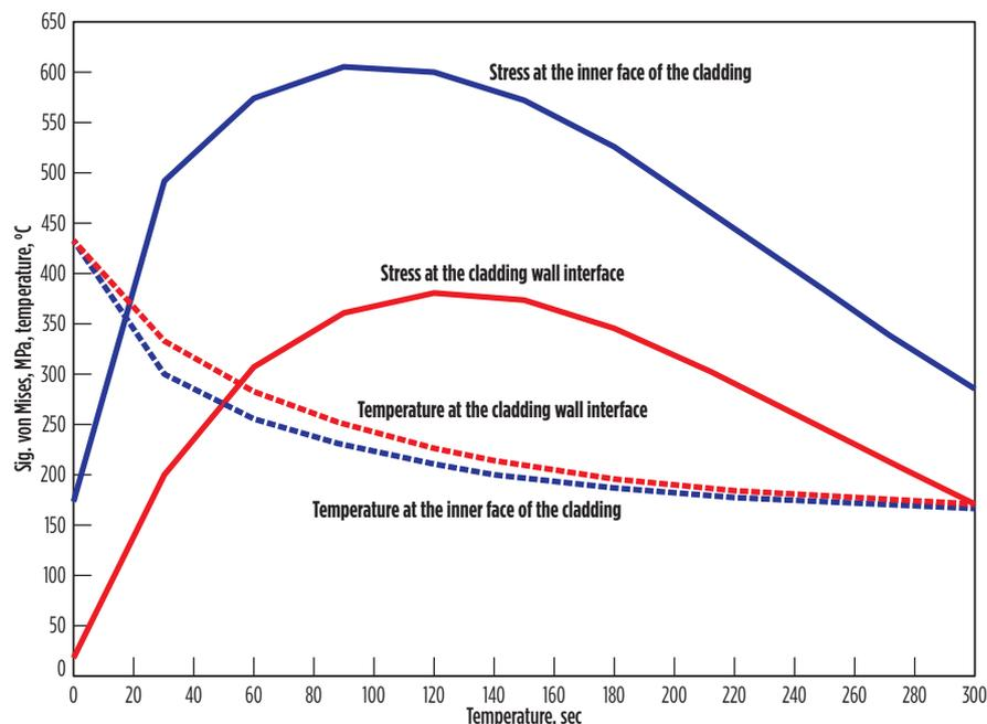
**FIG. 4.** Temperature and stress variation over time in the cladding during a thermal shock.
